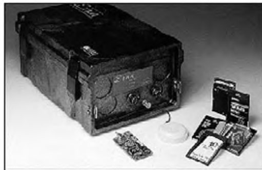
Figure 5.14. Example of a recorder made specifically for strong motion, the Kinematics Etna. The round white box in front of the recorder is the GPS antenna and the PCMCIA cards are seen to the right. From Kinematics home page www.kinematics.com .
