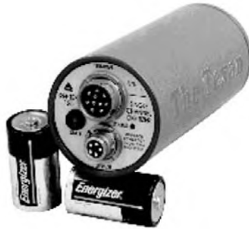
Figure 5.15 The RefTek Texan one channel recorder. From RefTek home page, www.reftek.com .
