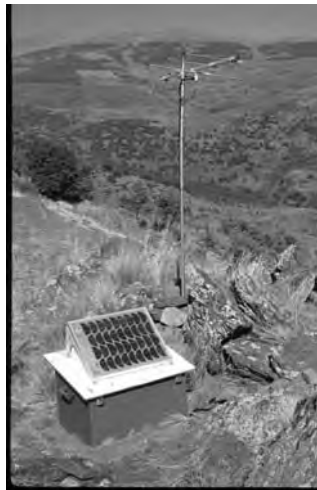
Figure 7.15 A small 12 W mono-crystalline solar panel mounted on top of the case of a temporary seismic station. Both sides of the panel are light sensitive, so the roof of the case is white-painted to reflect the diffuse radiation to the rear side of the panel.
