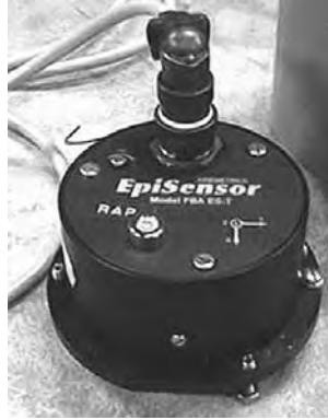
Figure 2.43 The Kinemetrics EpiSensor. The case contains a 3-component sensor. The diameter is 13 cm.
